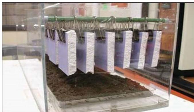
FIG. 1 Sample Holding Tank with Test Samples
